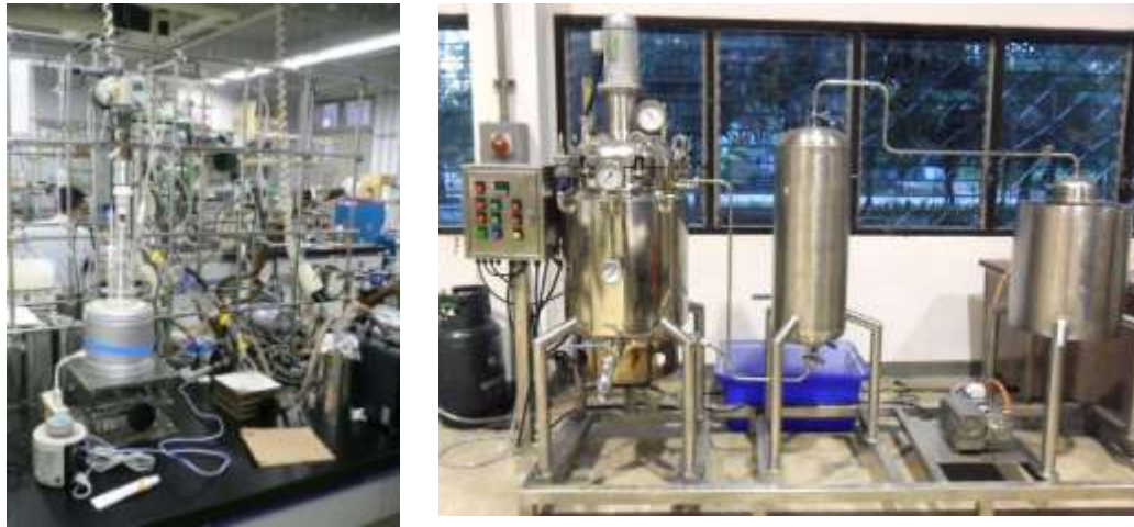
Fig. 1 Direct polymerization and pilot plant for PLA preparation (made in RMUTT).
