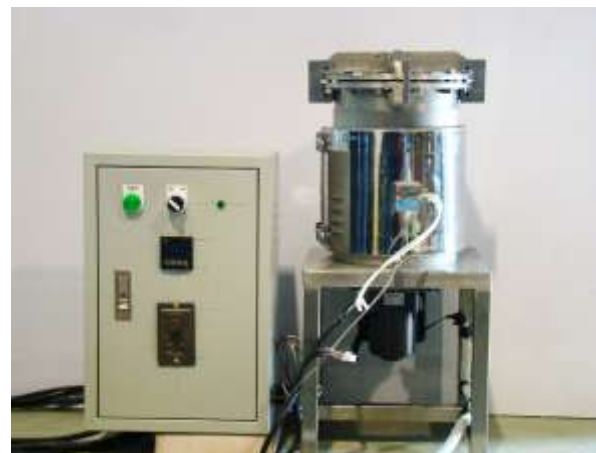
Fig. 2 Autoclave (made in RMUTT) for nanomaterials preparation.
