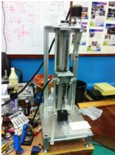
Fig.3 (left and right) Monofilament force test machine
